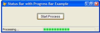
Figure 3. SFStatusBar combines a status bar and a progress bar in one control.
