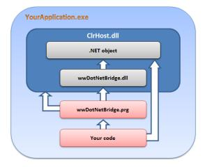
Figure 2. The architecture of wwDotNetBridge.
