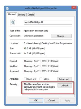
Figure 1. Unblock wwDotNetBridge.DLL to prevent errors when using it.
