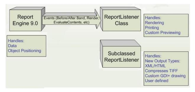
Report listeners produce output in two ways. "Page-at-a-time" mode renders a page and then outputs it. This is typically used when a report is printed.
