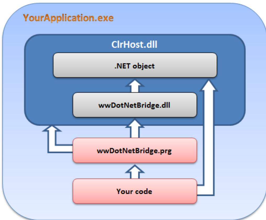
**Figure 3. The architecture of wwDotNetBridge.**
