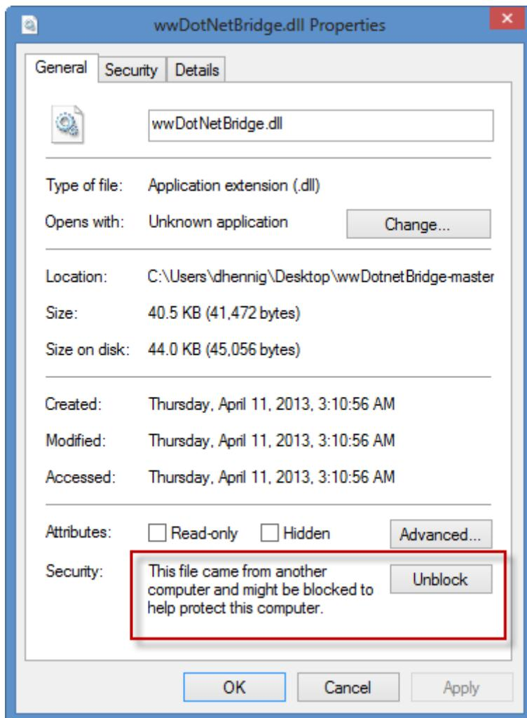
Figure 2. Unblock **wwDotNetBridge.DLL** to prevent errors when using it.
