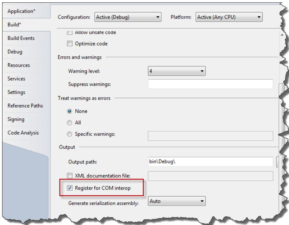
**Figure 1. Turn on "Register for COM interop" to automatically register the control on your system.**
