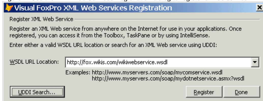
Figure 1. Use the XML Web Services Registration dialog to register a Web service in VFP.
