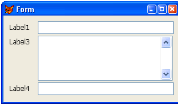
Figure 3. Turning off anchoring before moving the controls results in the proper placement.
