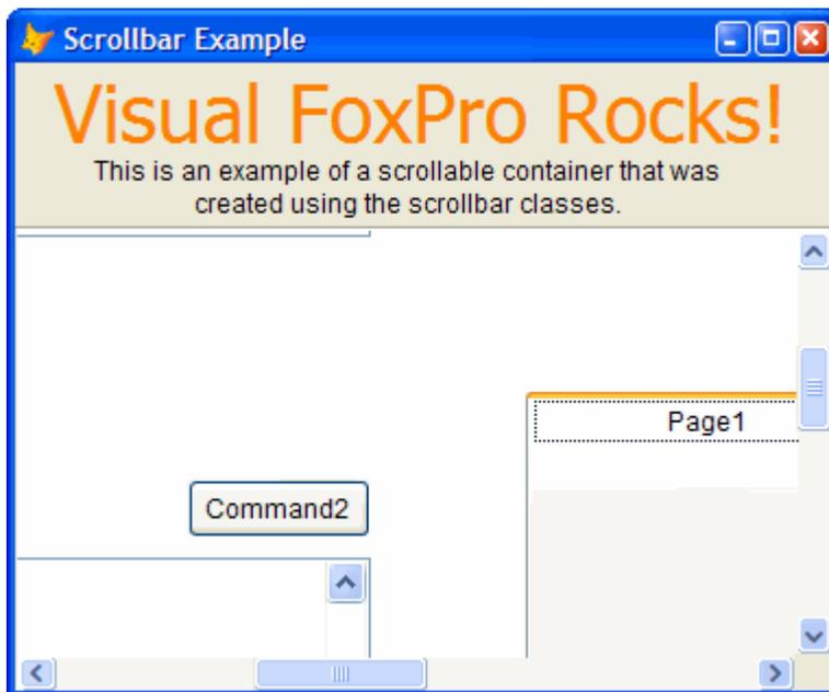
*Figure 3. The scroll bar control allows you to create a scrolling region in a form.*
