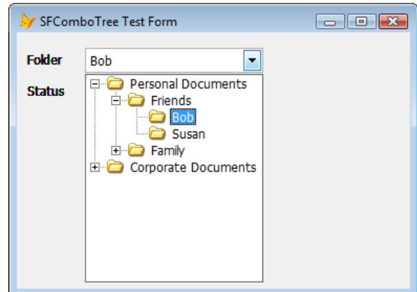
**Figure 2.** SFComboTree provides a combined combo box and TreeView control so the user can easily view a hierarchical list.
