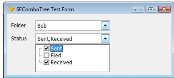
Figure 3. The second SFComboTree in the sample form demonstrates a list of items with checkboxes.
