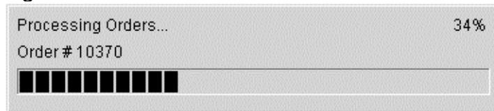
In addition to the ProgressBar control, SFTermometer has three labels: one for the “main” label (the overall job being done, such as posting transactions), one for the “current task” (a subset of the job, such as calculating totals), and one to show the current percentage complete. These labels allow you to show what stage the process is at. It also has a Cancel button that allows the user to cancel the process. We’ll see how that’s accomplished later.
