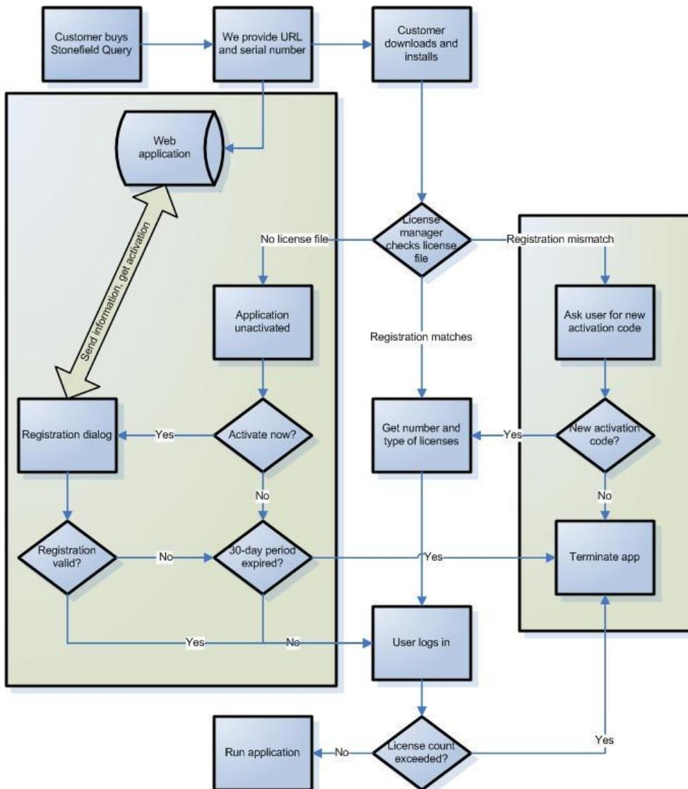
Figure 1. This flowchart shows the activation and licensing mechanism Stonefield Software uses.
