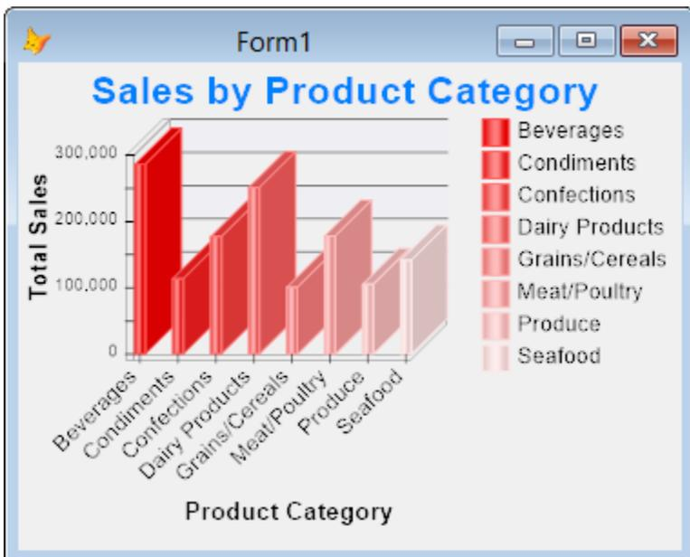
Figure 5. Setting ColorType to 3 and BrushType to 2 uses gradients.
