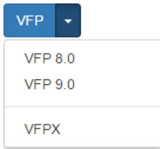
Figure 18. A split button acts like a button but includes a dropdown menu.
